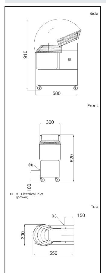
Electric Supply voltage: 220-240 V/1N ph/50 Hz **Electrical power, default:** 0.37 kW Capacity: Maximum kneading (60% hydratation): 8 kg/Cycle Key Information: External dimensions, Width: 300 mm External dimensions, 550 mm Depth: External dimensions, Height: 620 mm **Shipping weight:** 49 kg 10 lt **Bowl capacity:**
